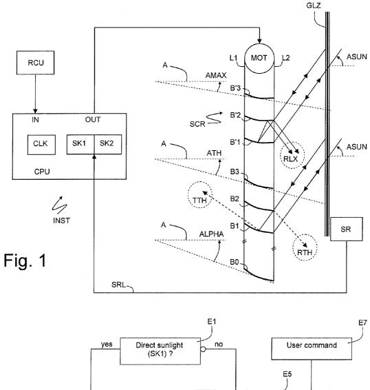
Strong luminance (SK2) ? yes E2 Automatically controlled Incline the slats to yes threshold ATH < another intermediate maximum aperture AMAX ? inclination E3 E4 Incline the slats to Incline the slats to automatically controlled threshold maximum aperture inclination AMAX Fig. 2 ATH
