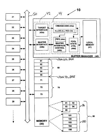
(57) Abstract: A method includes receiving a first buffer allocation command from a first processor, the allocation command including a register address associated with a pool of buffers in a shared memory, determining whether a buffer is available in the buffer pool based upon a buffer index corresponding to a free buffer, and if a buffer is determined available allocating the buffer to the first processor.
