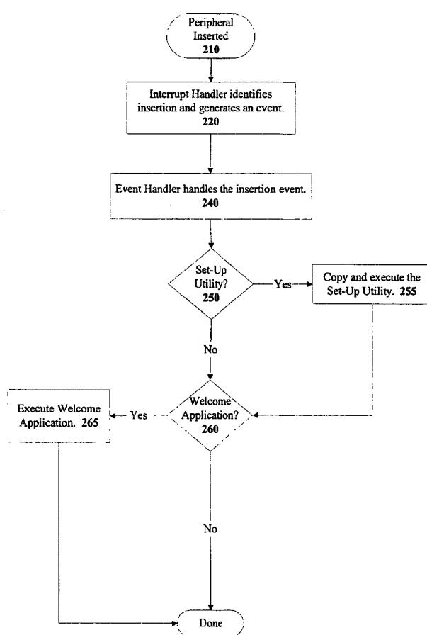
(57) Abstract: A robust external interface for a computer system is disclosed. The robust external interface allows a user to insert or remove external peripherals to the external interface at any time such that the user does not need to carefully follow any scripted procedures. The external interface software detects insertions or removals and acts in an appropriate manner.
