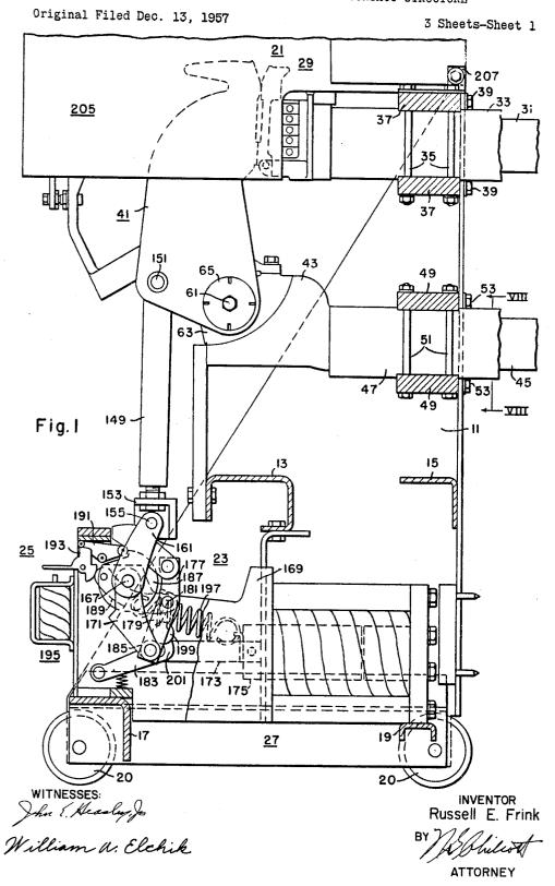
CIRCUIT BREAKER WITH IMPROVED CONTACT STRUCTURE
