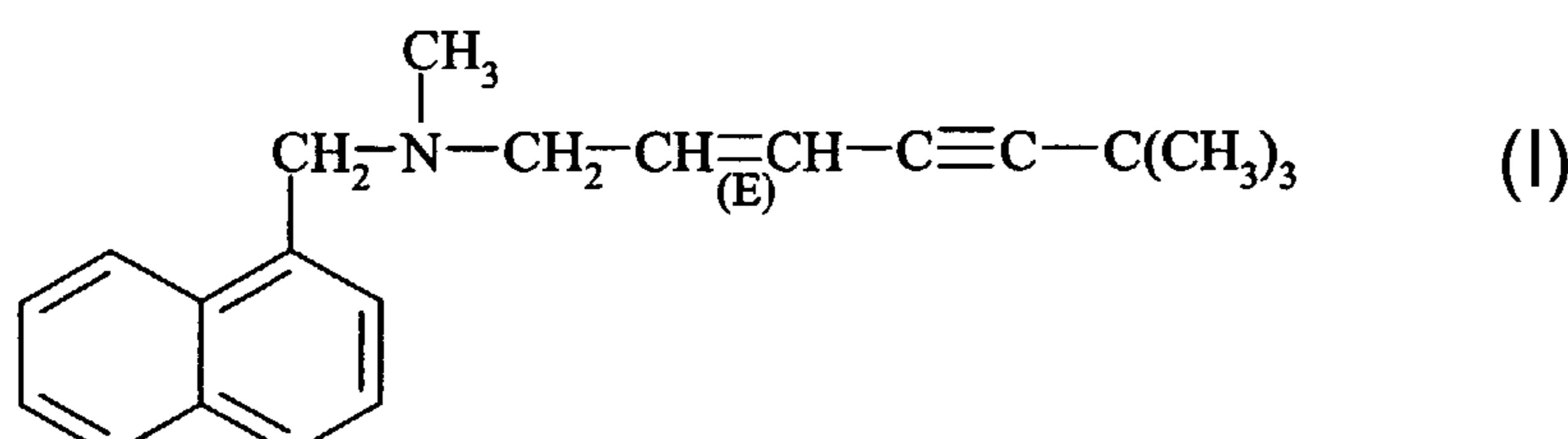
(57) Abstract: Purification process for the preparation of the allylamine pharmaceutical terbinafine of formula (I), in free base form or acid addition salt form, by distilling crude terbinafine base, preferably by short path distillation, e.g. at a temperature above 100°C and reduced pressure, e.g. 0.2 mbar, and recovering the purified
