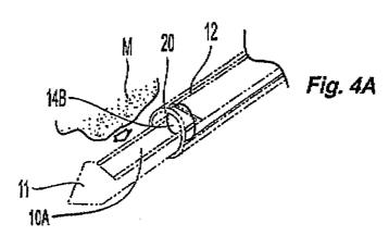
(57) **Abstract:** The present invention provides for exemplary embodiments of a single-insertion, multiple sampling biopsy device. Exemplary embodiments of a single-insertion, multiple sampling device with integrated marker release.
