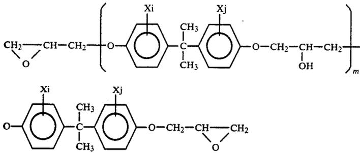
wherein X is bromine, i and j are each integers of from 1 to 4 and m is an average polymerization degree ranging from 0 to 40.
