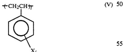
wherein X is a bromine atom, i is an integer of 1 to 4, and l is an average polymerization degree ranging from 0 to 40.
