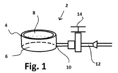
(57) Abstract: Ring-shaped cuff for being placed over the penis during circumcision and in order to release anaesthetic agent through a plurality of delivery zones under increased pressure to numb the dorsal nerves of the penis.
