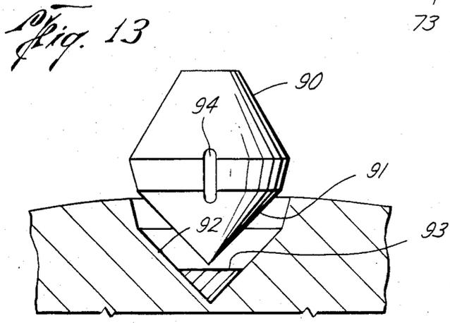
**DRILL BITS WITH CONE RETENTION MEANS**
