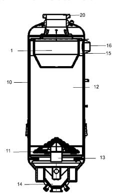
(57) Abstract: In the gasification of carbonaceous solids with oxygen and/or steam in a fixed bed, the reactor (10) operated under pressure must continuously be charged with the solids. These solids are supplied to the fixed bed (12) from a lock via a ring-shaped apron (1) open at the top and at the bottom. This apron (1) includes an inner and an outer jacket, so that a cooling gap is formed with at least one inlet and/or outlet for a cooling medium.
