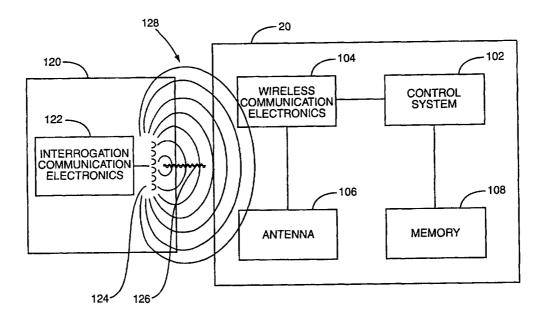
(57) Abstract: An identification device for providing information regarding a container to which the device is attachable, said device comprising: a wireless communication means containing said information; and a resilient member to which said wireless communication means is secured, said resilient member being attachable to the container by being deformable to conform to a portion of the container wherein attachment is caused by the resilience of the member.
