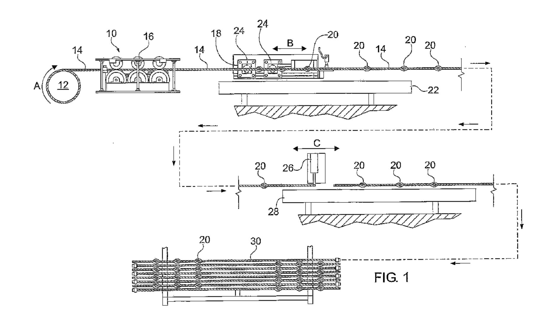
(57) **Abstract**: A method of forming a bulb in a cable bolt includes providing cable from a cable source, advancing the cable in a first direction, and forming a bulb in a portion of the cable while the portion of the cable is continuously provided from the cable source.
