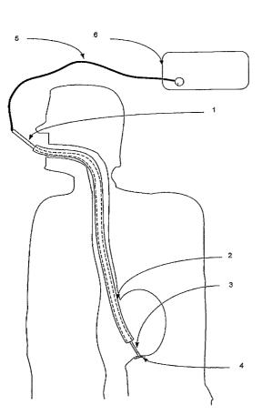
(57) Abstract: A flexible RF device (1) can be deployed through a flexible endoscope. An electrode structure has a central electrode (12) and outer electrode (11). Flexible electrodes (30), circular electrodes (51, 53) and circular loop assemblies (55, 56) with different diameters are also disclosed, as well a tweezer electrodes (41) with pads (43) for increasing contact area. Retractable electrodes (100) are also disclosed.
