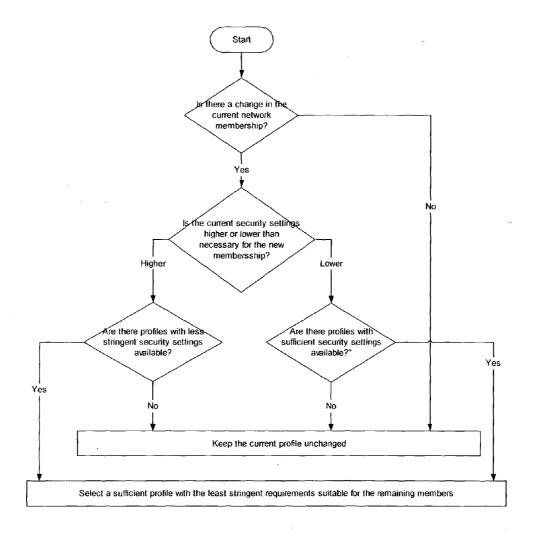
Figure 4 - Flowchart example of an adaptation rule to optimize throughput and security
