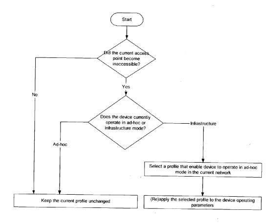
Figure 5 - Flowchart of a sample adaptation rule to optimize connectivity
