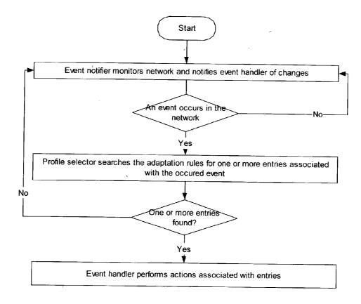
Figure 3 - Flowchart of the device adjusting the current operating profile to network changes
