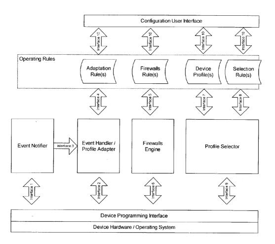
Figure 1 - An overview of components comprising the invention, and their interactions
