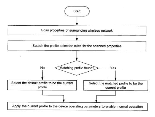
Figure 2 - Flowchart of the device joining or forming the wireless network
