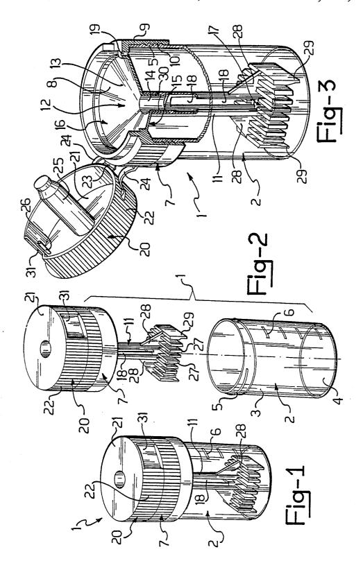
a funnel 15 which has an inlet mouth 16 open upwards and an outlet mouth 17 open toward the bottom 4 of the container.
