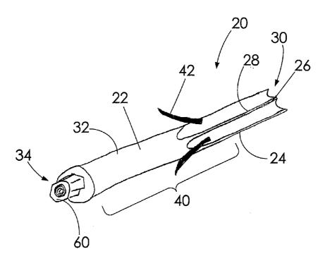
(57) Abstract: The present invention provides a device for treating fractures of a bone and methods for treating a facture, particularly fractures of the femur, that uses an intramedullary nail or a bone plate and a sliding compression fixation element. Certain features of various fixation elements described herein lessen the rotational forces applied during implantation and/or lessen the amount of bone that needs to be removed during placement of the sliding compression screw.
