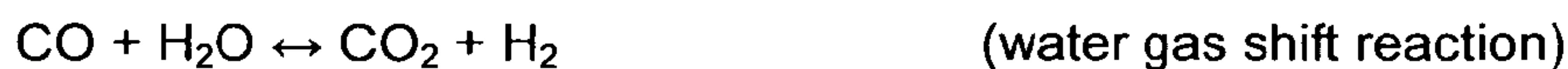
30 The reaction (1) has a stoichiometric ratio H<sub>2</sub>/CO of 1:1 and has some advantages over reaction (2). For example reaction (1) generally allows higher single pass conversions and less energy-consuming in comparison to the removal of water from the system in reaction (2).
