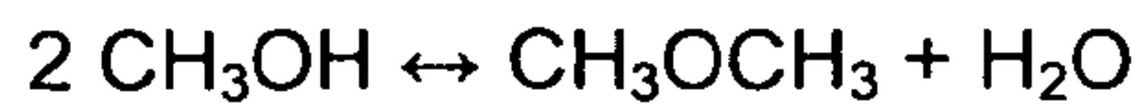
In the direct DME production there are mainly two overall reactions that occur from synthesis gas. These reactions, reaction (1) and reaction (2), are listed below.
