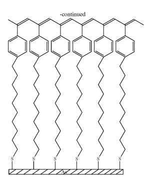
**[0063]** Example 3, above, illustrates a SAM of alkylphenylacetylene on an oxide insulating layer that has been polymerized by dipping in a solution of a catalyst, for example, a Ziegler catalyst, to form polyphenylacetylene at the surface of a polymerized SAM, which may form an intramolecular charge transport pathway between source and drain electrodes of a field-effect transistor.
