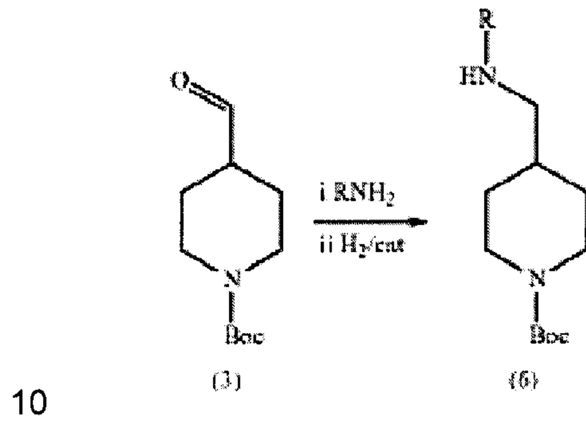
15 The corresponding amine (30 mmol) was added to a solution of 1-Boc-piperidine-4-carboxaldehyde (3) (30 mmol) in EtOH (40 ml) followed by 10% Pd/C (50% in  $\text{H}_2\text{O}$ , 0.3 g). The reaction was processed under a hydrogen atmosphere (40 psi) at room temperature until gas uptake finished and reaction completed (-2-3 hours). The reaction mixture was filtered through celite™ and the filtrate was evaporated to dryness to give product (6) in excellent yield.
