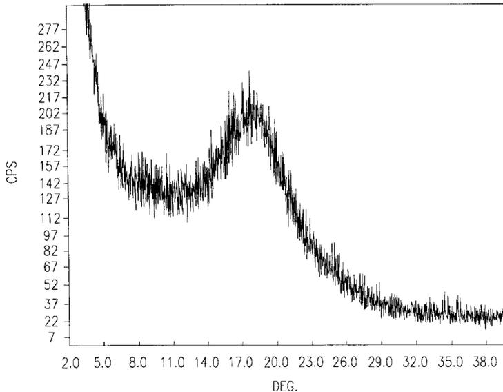
POWDER X-RAY DIFFRACTION PATTERN OF CRYSTALLINE COMPOUND OF FORMULA I
