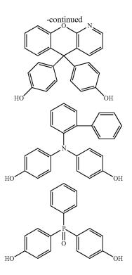
**[0132]** Dihydric phenol compounds of Formula (III) can be converted to a diepoxide using any suitable process and materials. The use of epichlorohydrin in the epoxidation process is presently preferred.
