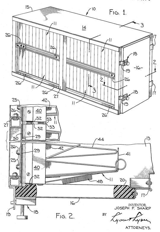
AIR FILTER ASSEMBLY WITH REMOVABLE FILTER ELEMENTS
