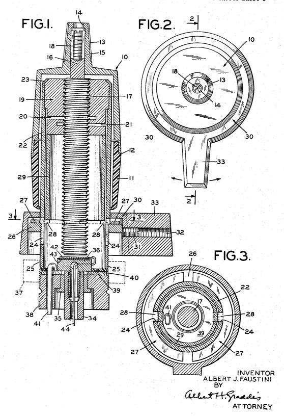
MICROMETER ADJUSTMENT LOCK
