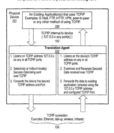
(57) Abstract: An architecture in which data outputs from an application program into a communication interface are diverted, by changing their address to a reserved address, and then are processed further by an added program which is invisible to the application program.
