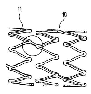
(57) Abstract: A medical device in the form of a stent (10) having struts (11) is disclosed. The stent (10) includes an outermost portion (43) having plurality of depressions (45) on the struts (11). The depressions (45) occupy at least about 80% of the surface area of the surface. The depressions (45) contain a coating material (77) that preferably includes a biologically active material and/or polymer where the outermost portion (43) is free of coating material (77).
