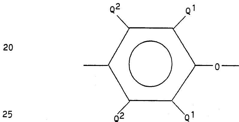
30 In each of said units independently, each Q<sup>1</sup> is independently halogen, primary or secondary lower alkyl (i.e., alkyl containing up to 7 carbon atoms), phenyl, haloalkyl, aminoalkyl, hydrocarbonoxy, or halohydrocarbonoxy wherein at least two carbon atoms separate the halogen and oxygen atoms; and each Q<sup>2</sup> is independently hydrogen, halogen, primary or secondary
