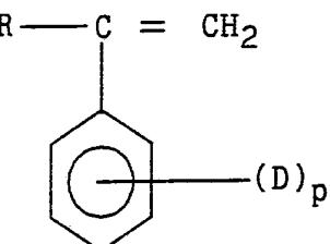
10 wherein R is hydrogen, lower alkyl or halogen, D is vinyl, halogen or lower alkyl, and p is from 0 to 5.
