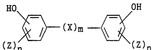
where (i) X is a substituted or unsubstituted, 30 linear or cyclic, divalent hydrocarbon radical containing 1-20 carbon atoms, or is a mixture of more than one of such radicals, or is -S-, -S-S-, -SO-, SO<sub>2</sub>-, -O-, -CO-, or a single bond; (ii) Z is independently hydrogen; a halogen such as fluorine, chlorine, bromine or iodine; or is a monovalent organic radical such as an alkyl group of 1-4
