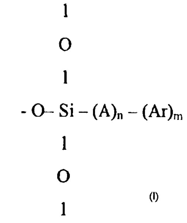
(57) Abstract: A high refractive index polysiloxane includes siloxane T units of the formula (I) where A represents an alkylene group having 1 to 4 carbon atoms: n=O or 1; m is at least 1; and Ar is an aryl group substituted by at least one iodine, bromine or chlorine atom, or is a polynuclear aromatic group. The invention includes chlorosilanes having the formula (Ar)m-(A)nSiCl3, useful in forming high refractive index polysiloxanes.
