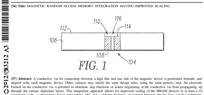
through the various deposited layers. This integration approach allows for improved scaling of the MRAM devices to at least a 45 nanometer node, a cell packing factor approaching 6F<sup>2</sup>, and a uniform thickness of material between the bit lines and the underlying memory elements.
