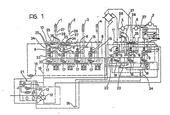
A flow recovery system for hydraulic circuits with pumps and pressurecompensated distributor valves for working members of earth-moving machines
