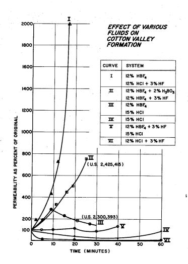
Fig. 1 I 2000 EFFECT OF VARIOUS FLUIDS ON COTTON VALLEY FORMATION 1800 **CURVE** SYSTEM 1600 12% HBF4 Ι 12% HCI + 3% HF 12% HBF4 + 2% H3BO3 1400 п 12% HBF4 + 3% HF 12% HBF4 Ш 1200 15% HCI 15% HCI 又 PERMEABILITY AS PERCENT OF ORIGINAL 12% HBF4 + 3% HF  $\mathbf{X}$ 1000 15% HCI 12% HCI + 3% HF VI 800 II e (U.S. 2,425,415) 600 400 (U.S. 2,300,393) 200 Ш  $\mathbf{v}$ V 100 **♣**∇I 40 50 20 30 10 0 TIME (MINUTES)
