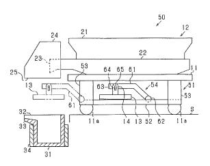
and a standby position located above a hood. When the furnace lid is in the standby position, the opening is open, and the melting material can be supplied into the crucible therefrom.
