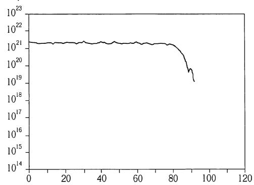
Depth of first phosphor layer measured by secondary ion mass spectrometer (nm)
