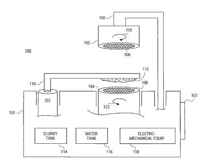
(57) Abstract: Conditioning of chemical mechanical planarization (CMP) using conventional diamond-embedded abrasive strips are well suited to condition conventional "hard" polishing but not soft polishing pads because the diamonds not only remove waste material, but they also damage the polishing surface of the pad. Embodiments of the present invention condition soft polishing pads using diamond strips without damaging the soft polishing pad (108).
