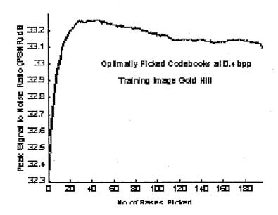
Figure 2 PSNR as successive bases are selected in a 14x14 separable codebook at a fixed rate of 0.4 bpp
