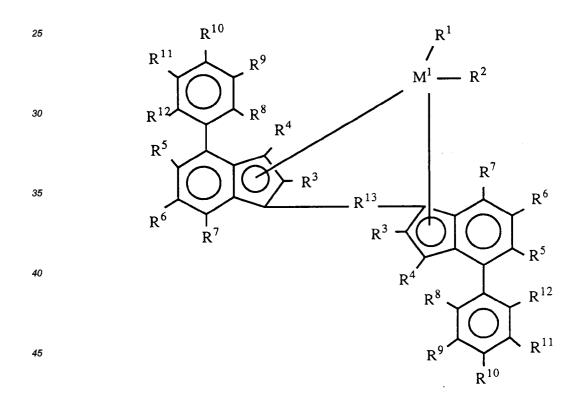
wherein M<sup>1</sup> is a transition metal atom, R<sup>1</sup> and R<sup>2</sup> are each a holagen atom, etc., R<sup>3</sup> is an alkyl group of 1 to 10 carbon atoms, etc., R<sup>4</sup> to R<sup>12</sup> are each an alkyl group of 1 to 10 carbon atoms etc., R<sup>13</sup> is a hydrocarbon group or a silicon containing group.
