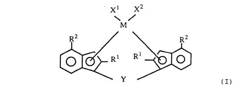
In the formula (I), M is a transition metal of Group IVa, Group Va or Group VIa of the periodic table. Examples of the transition metals include titanium, zirconium, hafnium, vanadium, niobium, tantalum, chromium, molybdenum and tungsten. Of these, titanium, zirconium and hafnium are preferred, and zirconium is particularly preferred.
