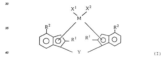
wherein M is a transition metal of Group IVa, Group Va or Group VIa of the periodic table; each R<sup>1</sup>, which may be identical or different, is a hydrocarbon group of 2 to 6 carbon atoms;
