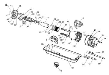
(57) Abstract: A linear compressor comprising a cylinder part (10) including a cylinder bore (71) and a piston (4) disposed in, And slidable within the bore (71). A main spring (15) connects the cylinder part (10) increding a dynamic state (1) and a slidable within the bore (71). A main spring (15) and the piston (4). A stator (5) has an air gap through which the connecting rod (47) passes. At least one armature pole (2) is located along the connecting rod (47).
