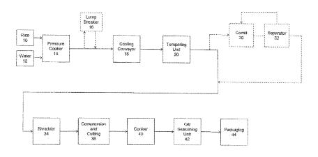
rice material, and shredding the tempered whole grain rice material to form continuous net-like sheets of the whole grain rice shredded product.
