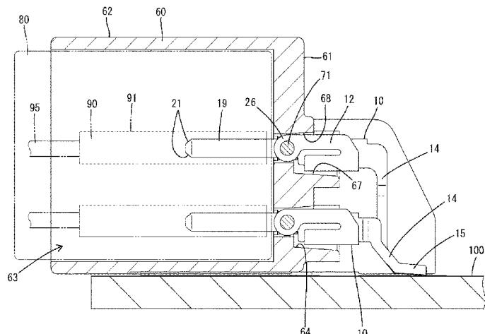
tion and the board connecting portion. The housing includes a supporting portion for rotatably supporting the terminal fitting by being engaged with the shaft portion. The terminal fitting has a center of gravity on a side closer to the board connecting portion than the shaft portion.
