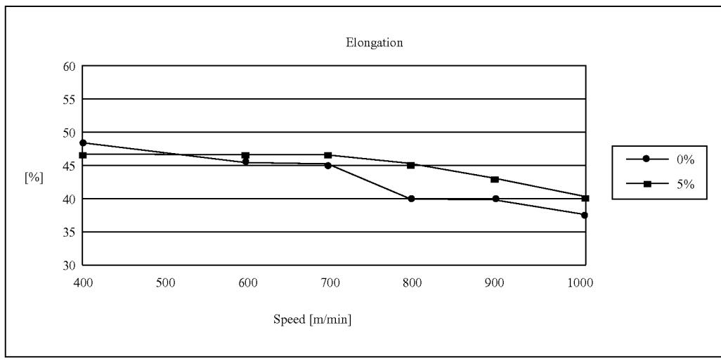
[0209] It is generally remarkable that texturing speeds of more than 400 m/min could be achieved. Compared to solution-dyed polypropylene, yarn tensile strength is so low from a pigmentation level of about 3% that the yarn breaks at high speeds. Consequently, doubling the texturing speed would significantly reduce these processing posts.
