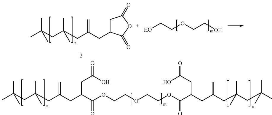
[0064] Here, n and m are, independently of one another, natural numbers. They are chosen by the skilled worker such as to give the molar masses defined at the outset for the hydrophilic blocks and the hydrophobic blocks, respectively.
