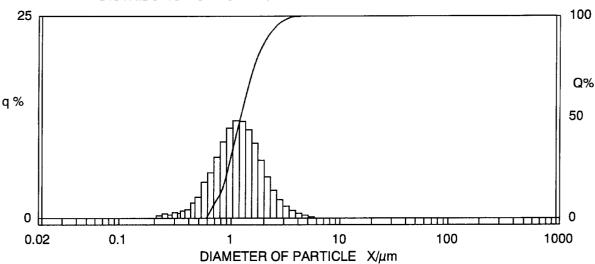
MEDIAN SIZE = 1.205μm SPECIFIC SURFACE = 12707cm²/cm² DIAMETER OF PARTICLE% (10.000 $\mu$ m) =100.0% %DIAMETER OF PARTICLE(90.0%) =2.239 $\mu$ m
