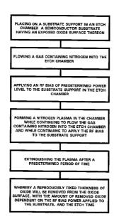
PLACING ON A SUBSTRATE SUPPORT IN AN ETCH CHAMBER A SEMICONDUCTOR SUBSTRATE HAVING AN EXPOSED OXIDE SURFACE THEREON
