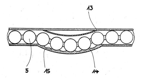
DEVICE FOR ADAPTING THE LENGTHS OF A PAIR OF LEGS, SUCH AS THOSE OF A LADDER, TO UNEVENNESS OF A SUPPORTING SURFACE
