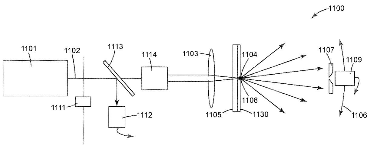
(57) Abstract: Microscatterometry system for generating an angularly resolved scattered light profile from the collected data.
