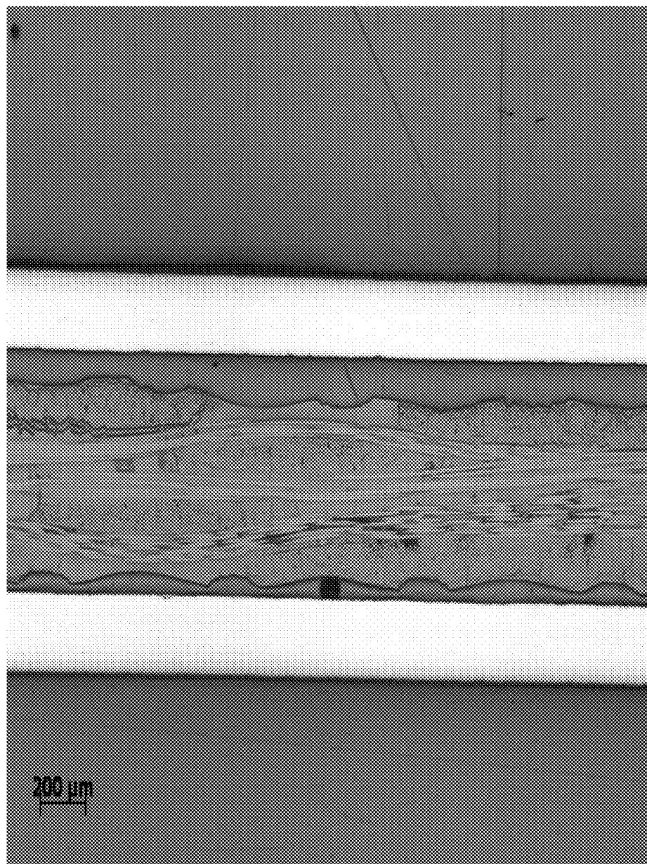
Fig 11. Oxide-oxide composite cross section 200micron
