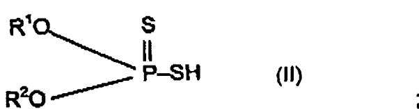
wherein R<sup>1</sup> and R<sup>2</sup> are independently hydrocarbyl groups of 6 to 18 carbon atoms; and wherein the acylated nitrogen-containing compound comprises a polyisobutene substituted succinimide having a TBN of 5 to 30, the polyisobutene substituent having a number average molecular weight in the range of 700 to 3000.
