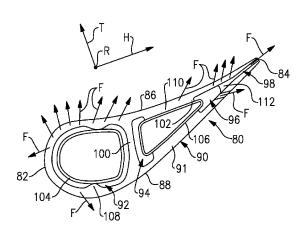
outer airfoil wall from the supply passage to the exterior surface on the suction side.
