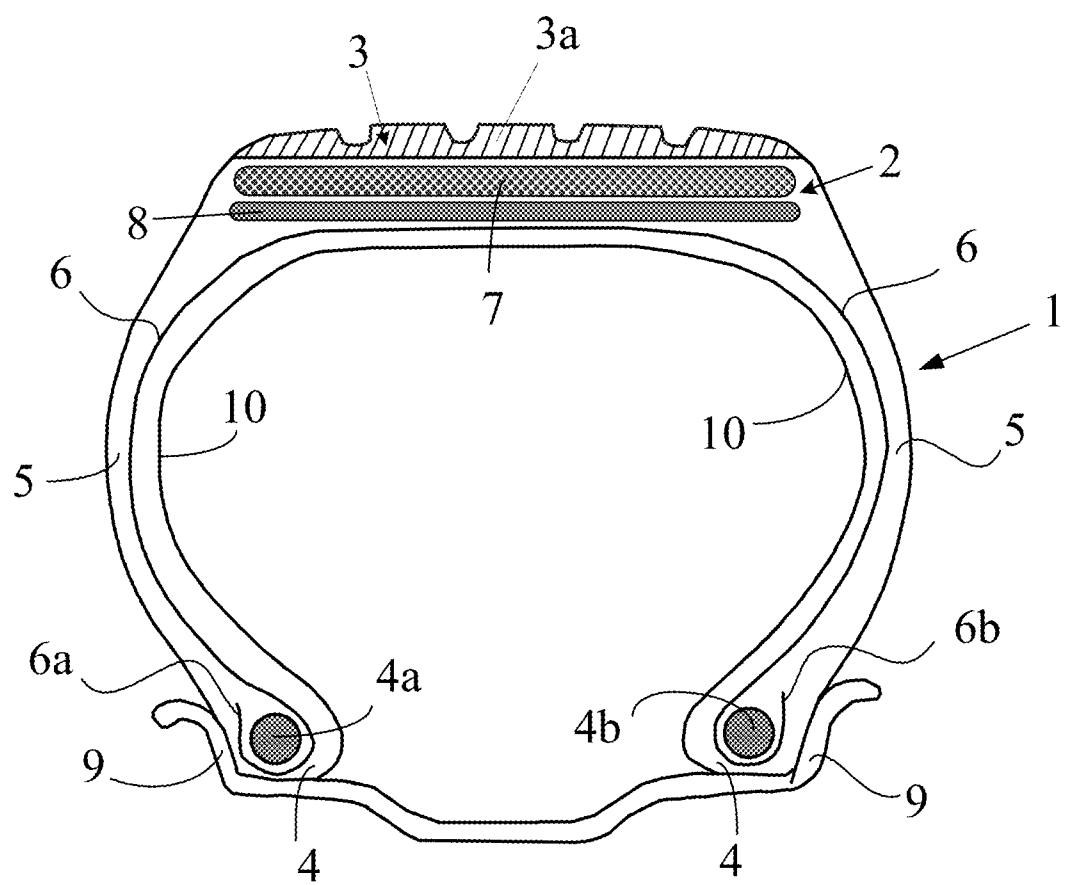
**TIRE, THE CROWN AREA OF WHICH IS PROVIDED WITH AN INNER LAYER FOR REDUCING RUNNING NOISE**
