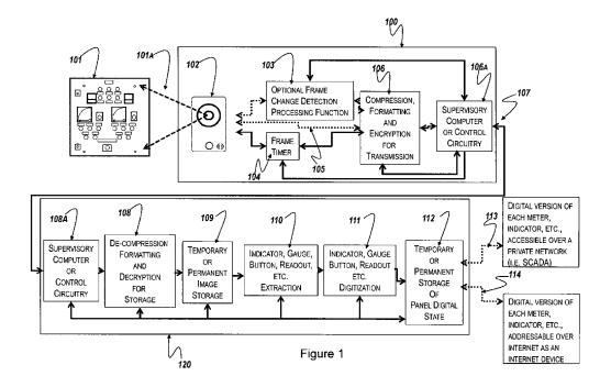
(57) Abstract: A system for digitizing gauges, lights and other human-readable machine gauges and functions and status without interfering with the operation of the machine or requiring reworking or interfering with the existing machine wiring, signaling, electrical or mechanical elements or operating modes, or adding new digitizing equipment to the machine.
