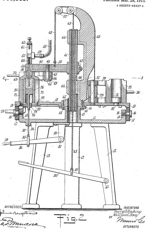
H. O. BISBING & W. L. 800Y. APPARATUS FOR MOLDING BOTTLES. APPLICATION FILED AUG. 6, 1910.
