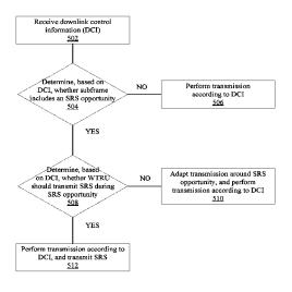
SRS transmission in the first subframe. If it is determined the WTRU is triggered to transmit the SRS transmission in the first subframe, the WTRU may transmit the SRS transmission on the SRS resources for the first subframe.
